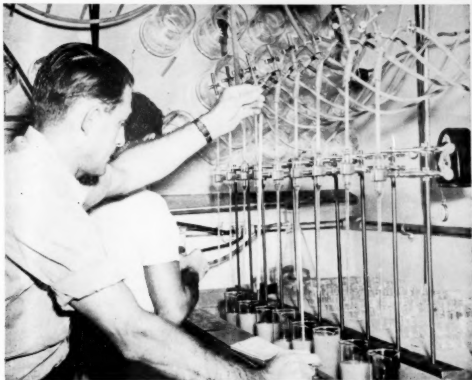
The pipette method of mechanical analysis for determining the sizes of the particles in a sample of sediment. The larger particles settle out faster, according to a known relationship. Aliquots are taken with the pipette at certain fixed times and depths, which establish the speed of settling and also show the size. The pipette aliquots are then dried and weighed. The weight of each sample is proportional to the percentage of material of the particular size. This photo shows a battery of 10 settling cylinders and pipettes, for turning out analyses in volume. The temperature is measured periodically during the run because the speed of settling depends partly on the temperature of the suspension. Photo by Wm. S. Russell.
